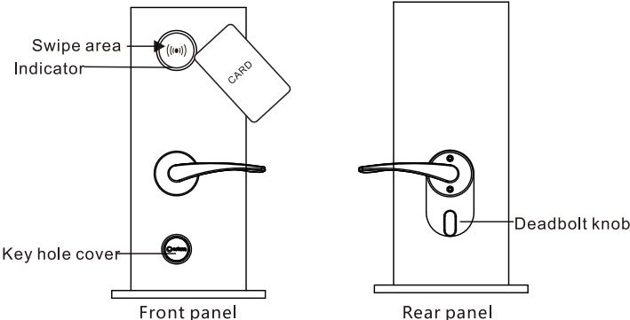
3-2: Lock from inside: Rotate the deadbolt knob on the rear panel for the double lock function (Note: The card needs to be encoded by the compatible management software and card encoder before use).
